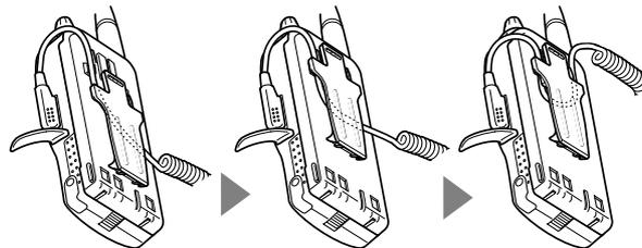
To remove the belt hook, pull the belt hook downward while pushing its tabs from both sides.
